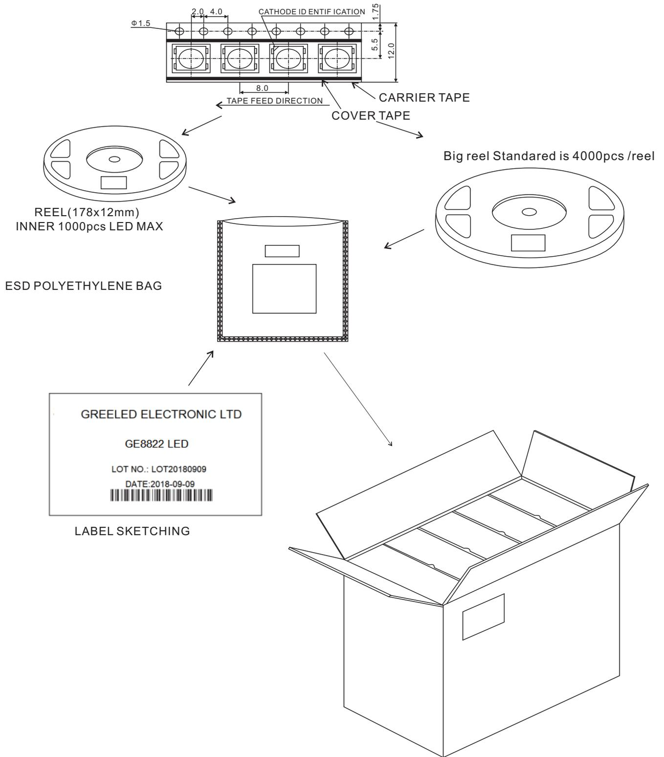
The reel pack is applied in SMD LED. The LEDs are packed in cardboard boxes after packaging in normal or anti-electrostatic bags. cardboard boxes will be used to protect the LEDs from mechanical shocks during transportation. The boxes are not water resistant and therefore must be kept away from water and moisture.
